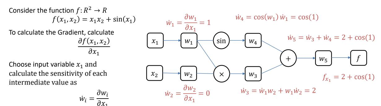
Accurate up to working precision, but still scales linearly in n.  $Cost(J_f) = n c Cost(f)$
